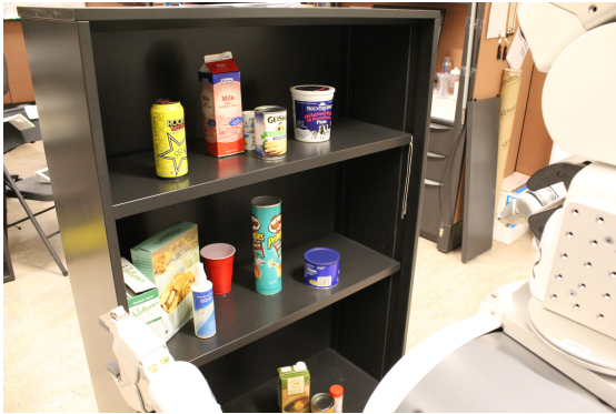
Fig. 4: Experimental setup. The PR2 with a head-mounted Kinect views the objects on a shelf from the front. The task is to search for a target object by rearranging other objects on the shelf.
