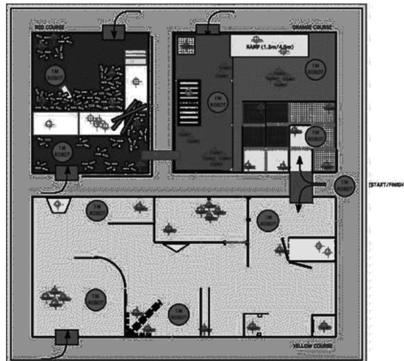
Fig. 6. Layout of the NIST Standard Test Course for USAR. Upper left box is the red section. Upper right box is the orange section. And the bottom rectangle is the yellow section.
