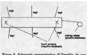
Figure 3: Schematic representation of Genghis, its positive and negative feedback sensors and its distributed collection of learning behaviors.
