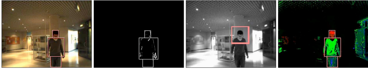
Fig. 3. Video feature maps with the 3-box body model superimposed. (a) Camera image, (b) Foreground segmentation. (c) Detector response. (d) Color segmentation (head–torso–leg color model projected to the red–green–blue channel, respectively).
