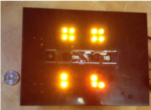
Figure 2: Prototype sensor package proposed in this work, consisting of an RGB-D sensor and amber LEDs. The camera and LEDs are covered with polarizing film oriented in perpendicular directions.
