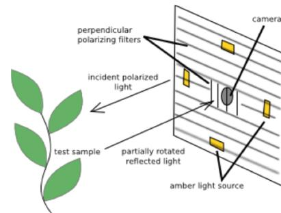
Figure 1: HLB detection methodology proposed by Pourreza et al. [17]. An array of high power amber LEDs with a polarizing filter illuminates the target leaves. A camera with a perpendicular filter measures intensity of rotated light.
