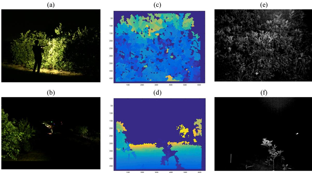
Figure 9: (a) Sensor in use for handheld sensing. (b) The sensor in flight. The UAV-mounted sensor was used to image trees in the orange grove from the side. Reset, or recently planted, trees were used as identifiers of healthy trees. (c) through (f) show images acquired by the RGB-D camera. Scaled depth images of (c) infected and (d) reset trees. Intensity images of (e) infected and (f) reset trees.
