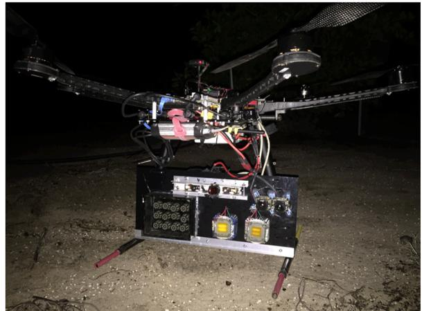
Figure 3: Updated sensor package, mounted on a DJI S800 hexacopter. Both a narrow-band amber and broad-spectrum light source were used. The broad-spectrum light source was processed through the red channel of the RGB-D camera. The sensor also consisted of two grayscale cameras and a 3DRobotics Pixhawk autopilot system.
