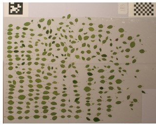
(b) Unwarped image after a perspective transform using the camera calibration board placed in the right top corner of the table.
