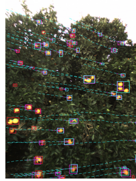
(b) Fruit detection and tracking is carried out simultaneously to generate a running count of fruits along a row. The red boxes show detection of new fruits, the cyan boxes show new fruits that were counted in the frame. The cyan lines show the paths of a detected fruit from previous images into the current image. The purple boxes show predicted positions of the fruits detected in previous frames.
