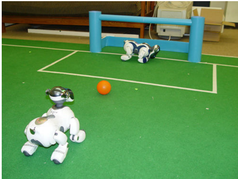
Figure 5.3: The setup for each run of the penalty kick-type experiment testing both shoot on goal behaviors
