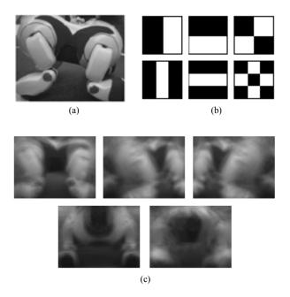
Fig. 4 (a) An example side view image used when creating the mean image for the side view model. (b) The six feature masks defining the rectangular regions whose mean pixel intensities were used to create features that enabled comparison between the model images and hypothesis windows. (c) The five robot models used in the approach, each representing a possible view of the robot, which are: side, angled right, angled left, front, and back.
