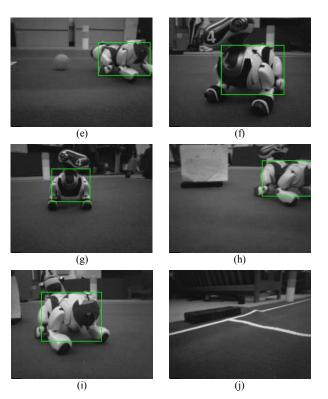
Fig. 7 Results of the combined robot detector which combines the color segmented image object detection method with the grayscale image robot classifier
