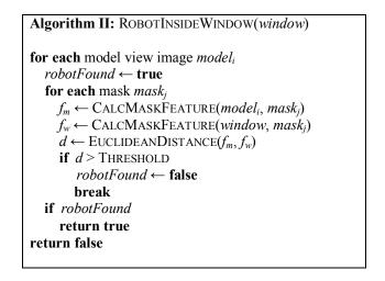
Fig. 3 Algorithm for classifying whether or not robots are contained within the given grayscale image window.
