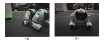
Fig. 6 Failure cases with combined detector. (a) False positive on the left. (b) False negative on robot, with initial hypothesis shown.
