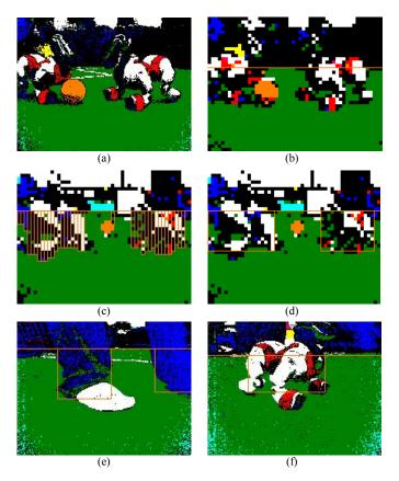
Fig. 2 Illustrative procedures and example results of the color segmented image object detection method. (a) Initial color segmented image. (b)Reduced image with detected field horizon. (c) Initial column scan results for object colors. (d) Final detected objects after grouping columns. (e) Detection result for a person's legs. (f) Detection result for an AIBO on the field.
