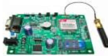
Fig 2. GSM modem used in the robot
