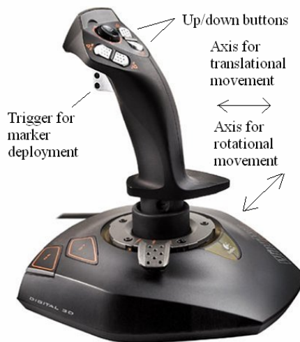
Figure 4: Joystick interface for teleoperated blimp control
