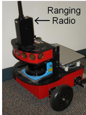
Figure 2: Photograph of Multispectral ultra-wideband ranging radio mounted on Pioneer robot. The robot was teleoperated around the environment to act as the moving target.
