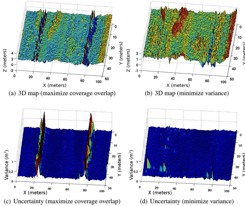
**Fig. 4** 3D bathymetric reconstructions found using sidescan sonar (top) and accompanying variance maps (bottom). Left: reconstruction resulting from dive patterns that maximize overlap in sensor coverage. Right: reconstruction from dive patterns that minimize the expected variance in a Gaussian Process representation of the reconstruction. The right image does not suffer from erroneous valleys that result from data sparsity, and the variance map matches this qualitative observation.
