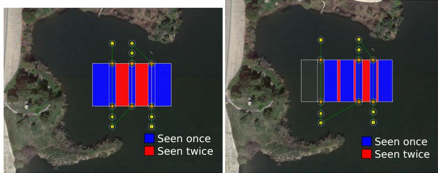
**Fig. 3** Dive patterns optimized to maximize coverage overlap (left) and uncertainty reduction (right). The region of interest is the  $100\text{ m} \times 50\text{ m}$  area (Lat.  $34.088854^\circ$ , Lon.  $-117.810667^\circ$ ) surrounded by the rectangular sensor footprint and highlighted in blue and red. Points of interest covered once by the sidescan sonar are labeled blue (darker), and areas of interest covered twice are labeled red (lighter).
