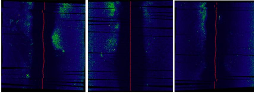
**Fig. 2** Example sidescan sonar images providing bathymetry information in Puddingstone Lake. Variations in the lakebed topography are apparent as bright returns in the images. A full 3D reconstruction can be found using shape-from-shading methods that make assumptions on the reflectance properties of the sonar.
