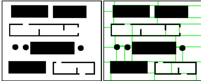
**Fig. 2** Polygonal representation of MAGIC environment (left) and discretization using a region growing technique (right).
