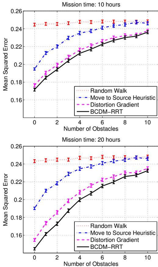
Fig. 2. Comparison of the BCDM-RRT sampling-based motion planning algorithm to a gradient-based approach and two heuristic strategies in a  $10 \text{ km} \times 10 \text{ km}$  environment with obstacles. The simulated vehicle is capable of unconstrained motion at a maximum speed of  $1 \text{ km/hr}$ . The proposed method provides improved estimation of the source signal for a given trajectory length. Each data point is averaged over 1000 random sensor deployments, and error bars are one SEM.
