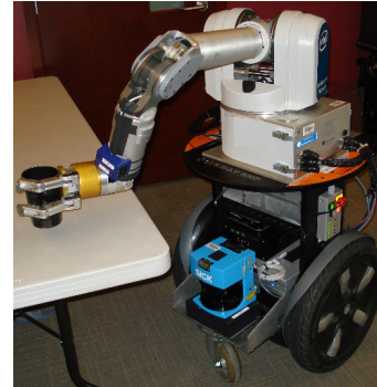
Fig. 1. Mobile manipulator: Segway RMP200 base with Barrett WAM arm and hand. The robot uses a wrist camera to recognize objects and a SICK laser rangefinder to localize itself in the environment
