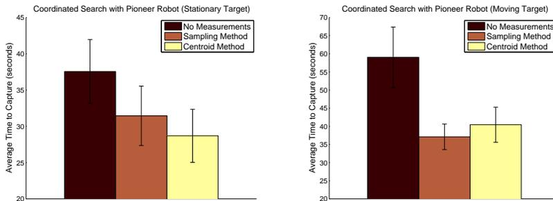
**Fig. 4.** Coordinated search results on a Pioneer robot comparing two methods for incorporating range measurements. Graphs show average capture times for a single searcher finding a stationary target (left) and a moving target (right). Error bars are one SEM, and averages are over 24 trials. Graphs are zoomed in for comparison.
