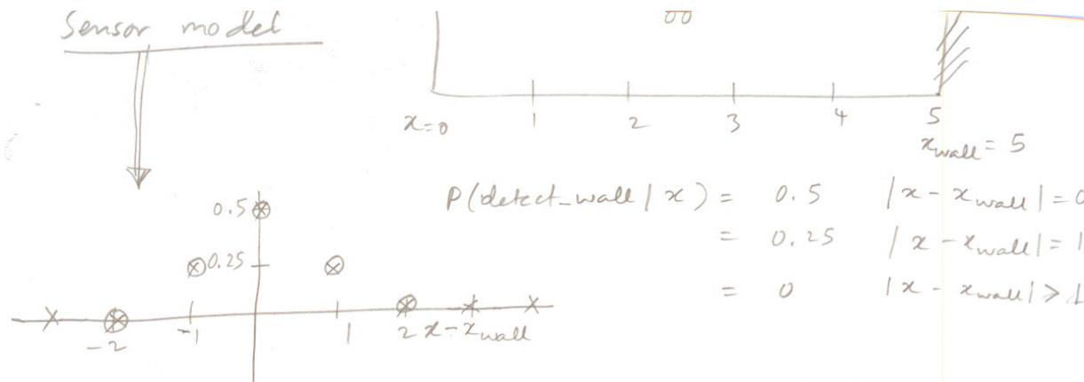
$$P(\text{detect\_wall} | x) = \begin{cases} 0.5 & |x - x_{\text{wall}}| = 0 \\ 0.25 & |x - x_{\text{wall}}| = 1 \\ 0 & |x - x_{\text{wall}}| > 1 \end{cases}$$
