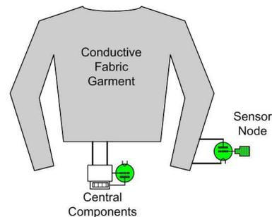
**Figure 1. Schematic of System Components Proposed by the Authors**
