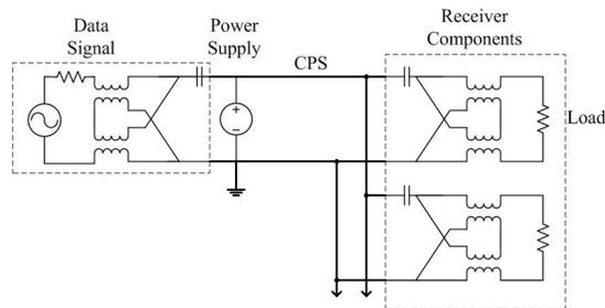
Figure 2. DC PLC System Diagram
