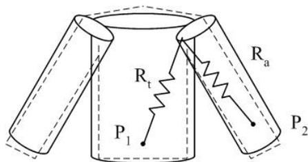
**Figure 6. Model for Predicting DC Resistance**
