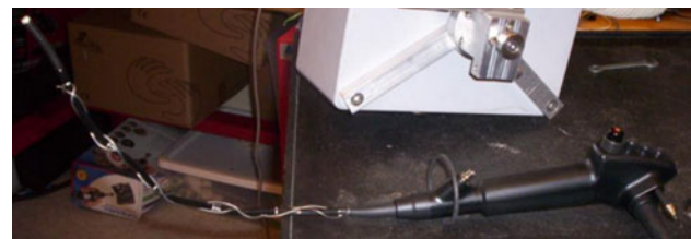
Fig. 2 The malleable support allows the scope shaft to stand up against gravity
