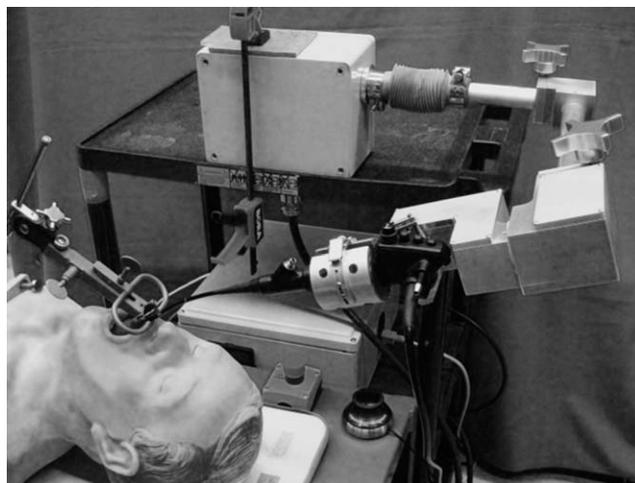
Fig. 2. The robotic endolaryngeal flexible scope mounted to a cart with an airway phantom. Controlling joystick is present in the mid-lower portion of the photo.
