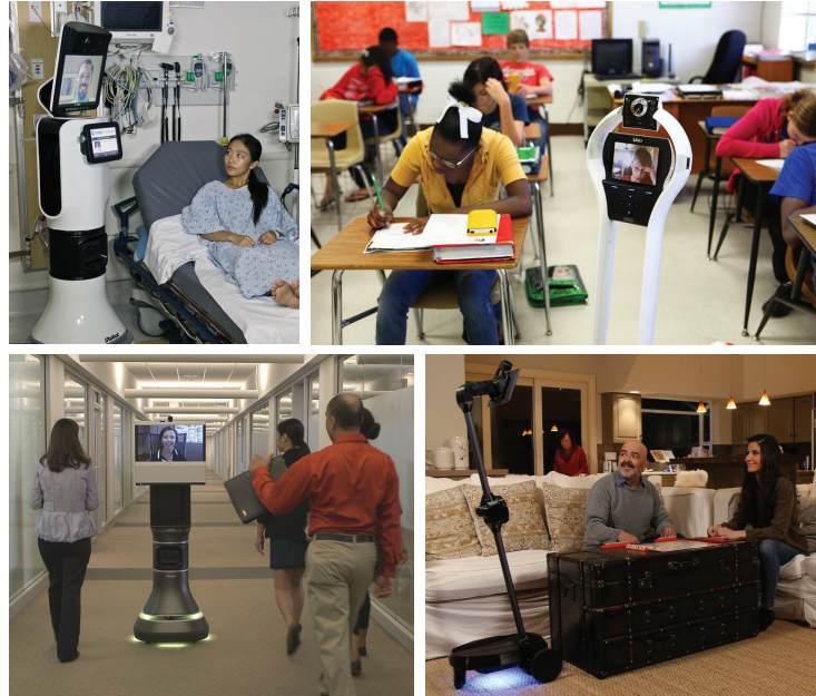
Figure 3.5: Telepresence robots, such as the RP-Vita, Vgo, AVA 500, and Ohmni (clockwise), are enabling robot-mediated communication in remote environments for human operators in settings such as hospitals, schools, offices, and homes.
