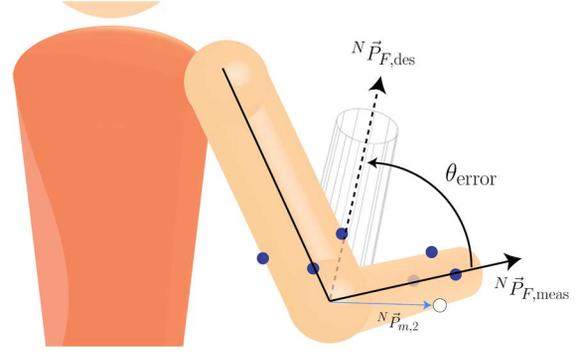
Fig. 4. Sample schematic illustrating the vectors used to calculate joint angle errors and which actuator is used to guide the user. In this example, to guide the user from their measured forearm orientation  ${}^N \vec{P}_{F,meas}$ , to the desired orientation,  ${}^N \vec{P}_{F,des}$ , the motor represented by the vector  ${}^N \vec{P}_{m,2}$  would be activated. This motor is colored in white to indicate that it is active.
