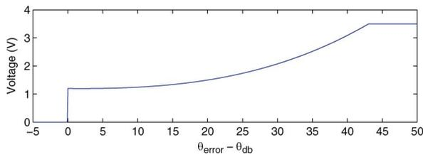
Fig. 5. Voltage commanded to the vibrotactile actuators as a function of the angle error outside the deadband. When the angle error was within the deadband, zero voltage was applied.
