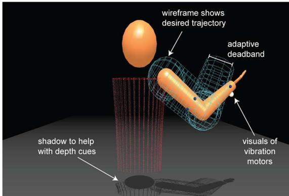
Fig. 6. Annotated screenshot of the visuals provided. User's own motions were displayed with an avatar. Wireframe arm, whose diameter was proportional to the deadband, indicated a desired trajectory. Users were instructed to stay within this region. Small spheres representing the vibrotactile actuators and a shadow on the virtual floor provided additional cues.
