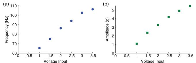
Fig. 3. (a) Frequency and (b) amplitude of vibration actuators as applied voltage increases.
