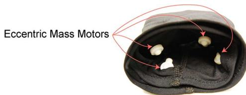
Fig. 2. Plastic caps (in white) are used to attach four vibrotactile actuators around the circumference of an arm band with equal spacing.
