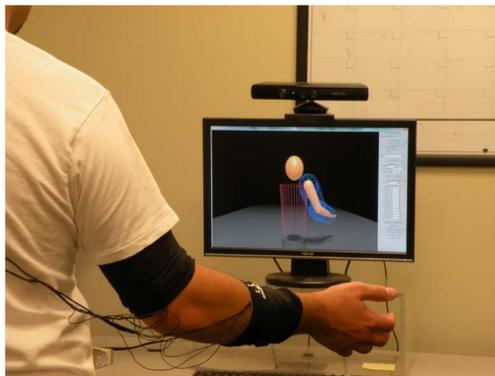
Fig. 1. StrokeSleeve tactile motion guidance system consists of a Microsoft Kinect to track the user’s motions, a computer screen to provide visuals of the measured and desired motions, and a pair of vibrotactile arm bands to indicate motion errors.
