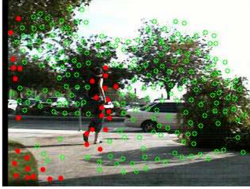
Figure 3.5: Outlier feature detection: Outliers are marked in red, filled circles, and inliers are marked in green, empty circles.
