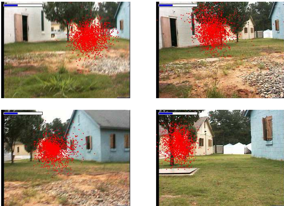
Figure 3.14: Snapshots of particle filter tracking a moving object: from Pioneer2 AT
