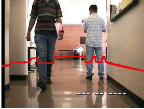
Figure 3.10: Projected laser scans: The image pixels at the same height as the laser rangefinder have depth information.
