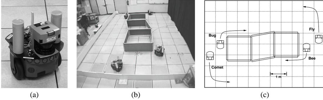
**Figure 3:** (a) A Pioneer 2DX equipped with a SICK LMS200 scanning laser range-finder and a pair of retro-reflective totem-poles. (b) The arena for the experiment; the central island is constructed from partitions that can be re-arranged during the course of the experiment. The dimensions of the environment are  $7\text{m} \times 5\text{m}$ . (c) Robot behavior: robots Fly and Comet follow the outer wall, robots Bee and Bug follow the inner wall(s).
