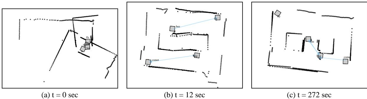
**Figure 4:** Experimental snap-shots. Each sub-figure shows the estimated pose of the robots at a particular point in time, with the corresponding laser scan data overlaid. Arrows denote the observation of one robot by another. Note that these are snap-shots of live data; they are not cumulative maps of stored data.
