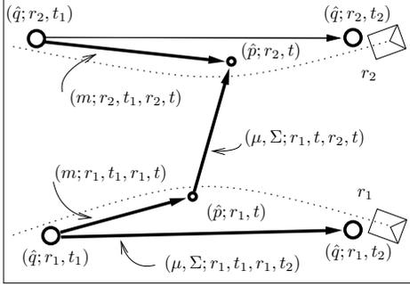
**Figure 2:** An illustration of the extended formalism. The figure shows two robots,  $r_1$  and  $r_2$ , traveling from left to right and observing each other exactly once. The robots’ activity is encoded in the graph, with nodes representing pose estimates and arcs representing observations. Also shown are the interpolated pose estimates  $\hat{p}_1$  and  $\hat{p}_2$  for each of the robots at time  $t$ .
