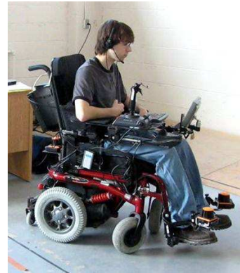
Figure 2–1: Autonomous Wheelchairs developed at McGill and Ecole Polytechnique de Montreal. These represent standard electric wheelchairs modified with onboard computing and sensing to allow for intelligent control.
