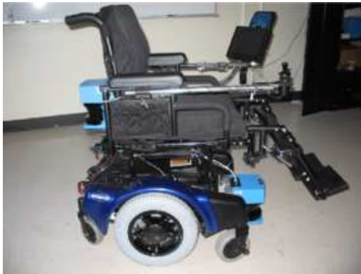
Figure 2–1: Autonomous Wheelchairs developed at McGill and Ecole Polytechnique de Montreal. These represent standard electric wheelchairs modified with onboard computing and sensing to allow for intelligent control.
