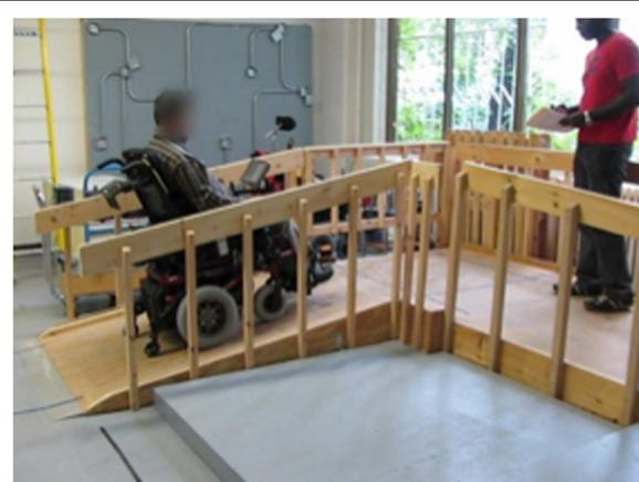
**Figure 10** Example of maneuver executions: slope climbing.
