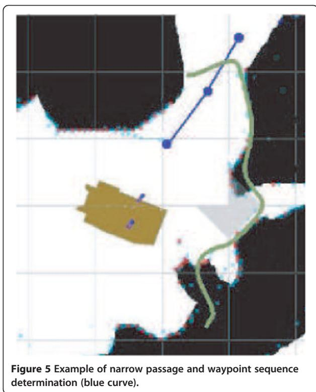
**Figure 5** Example of narrow passage and waypoint sequence determination (blue curve).
