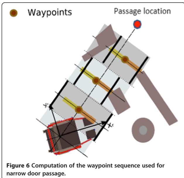
**Figure 6** Computation of the waypoint sequence used for narrow door passage.
