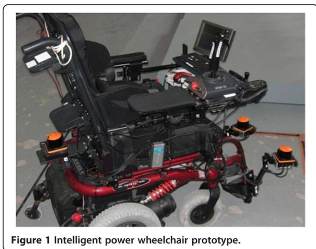
**Figure 1** Intelligent power wheelchair prototype.
