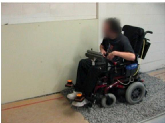
**Figure 12** Example of maneuver executions: motion on gravel.
