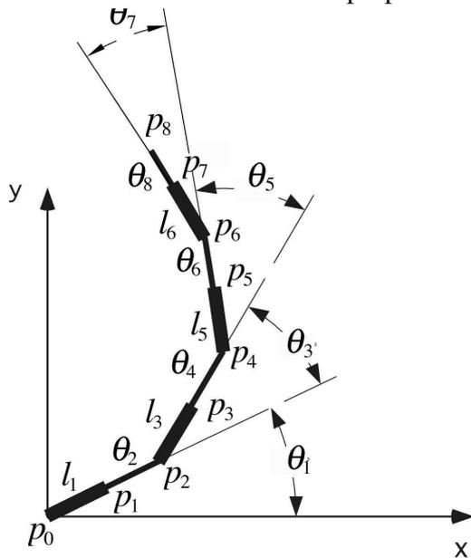
inverse dynamics model in the control loop such that desired states and current states always coincide). Details of the robot arm are in the figure below: it has one revolute joint followed by a prismatic joint, and so on. For simplicity, the joints have no stops, i.e., revolute joints can rotate more than 360 degrees, and prismatic joints can be positive or negative length.
