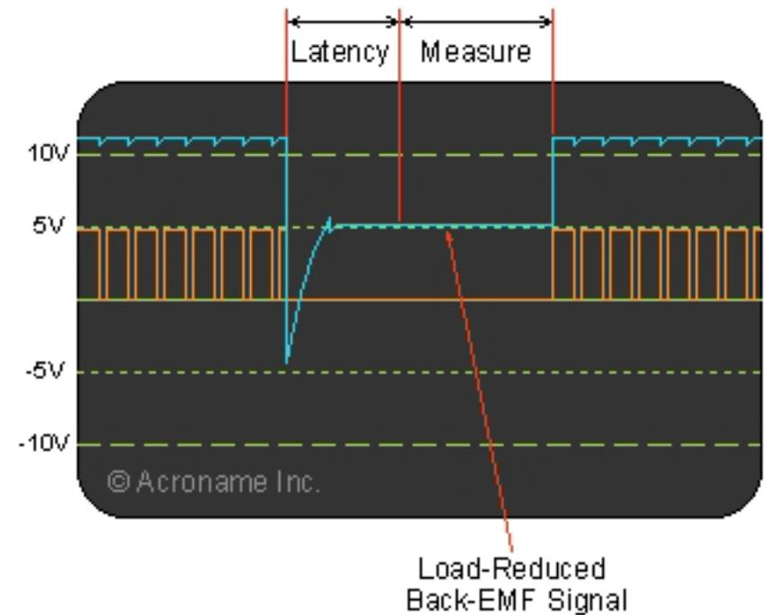
75% Duty Cycle with High Load Simulated Scope
