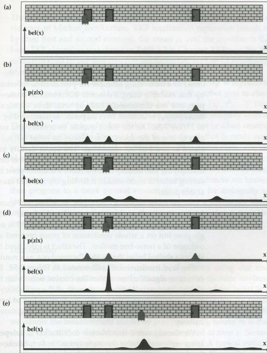
Figure 7.5 Illustration of the Markov localization algorithm. Each picture depicts the position of the robot in the hallway and its current belief  $bel(x)$ . (b) and (c) additionally depict the observation model  $p(z_t | x_t)$ , which describes the probability of observing a door at the different locations in the hallway.
