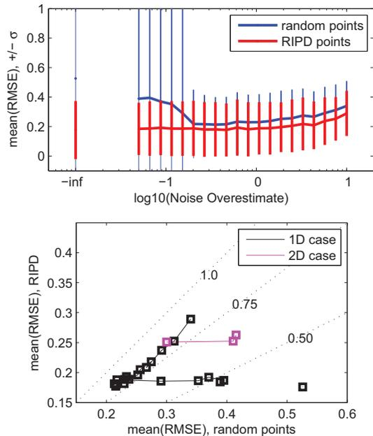
Fig. 2. DCT results summary. *Top*: 1D case, mean values of the random-point and RIPD ensembles, along with lines showing plus and minus one standard deviation for the ensemble, as a function of  $\hat{\nu}/\nu$ ; the leftmost point represents  $\hat{\nu} = 0$ . *Bottom*: Alternate view of the mean values above for one dimension, and three similar points for two-dimensional case with  $\hat{\nu}/\nu = [0, 0.05, 1]$ , right to left.
