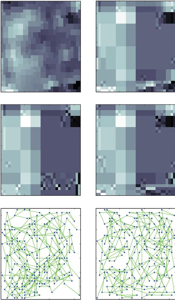
Fig. 3. *Top left*: Discretized image of a sea-surface temperature map. *Top right*: The sparsified SST map with  $S=50$ . *Middle left*: Typical reconstruction result using 200 points randomly selected, with maximum move 10 pixels. *Middle right*: Same for 200 RIPD points; the RMSE is 15% less than for random points. *Bottom left*: Random path associated with the reconstruction above. *Bottom right*: Same for RIPD path. *Note*: the bounding box drawn is outside the feasible set of points.
