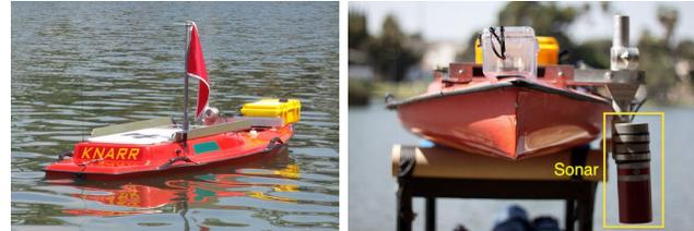
Figure 1. The USC ASV. Left: The ASV in operation in Echo Park Lake. Right: The ASV on shore with the sonar mounted.
