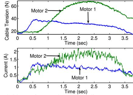
Fig. 2: Cable tensions and corresponding motor currents during example move
