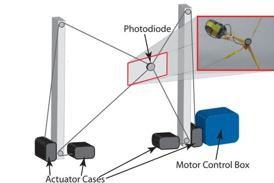
Fig. 1: Schematic of a NIMS-PL system actuating an optical sensor in a vertical plane while observing light intensity
