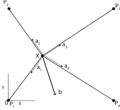
Fig. 3: Kinematic diagram of a NIMS-PL configuration showing  $\vec{a}_i$ ,  $P_i$ ,  $X$ , and an example desired force vector,  $\vec{b}$
