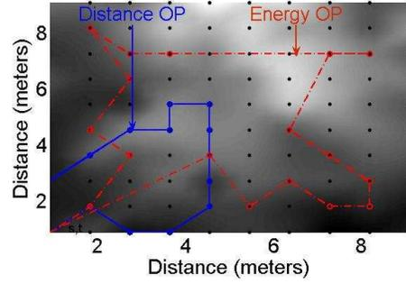
Fig. 6: Comparison of paths found using DOP and EOP for the initial budget constraint of 16 meters for Euclidean distance cost model
