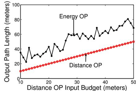
Fig. 7: Comparison of distances traveled by the DOP and EOP methods while expending equal total energy
