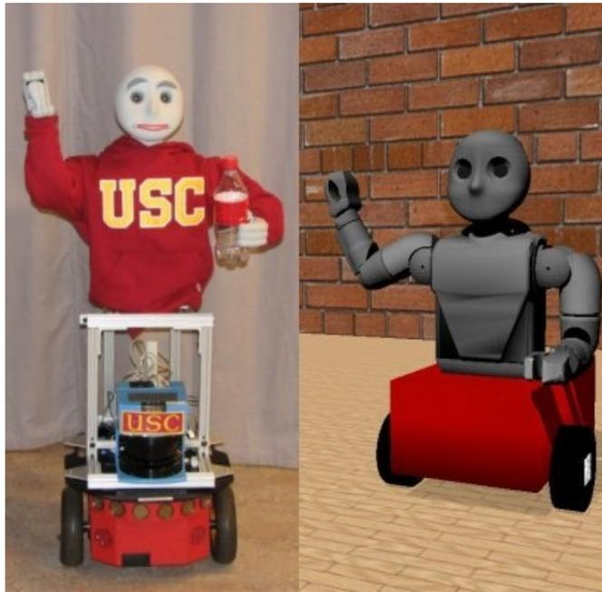
Figure 1: An example of an HRI testbed: a humanoid torso on a mobile platform, and a simulation of the same system.
