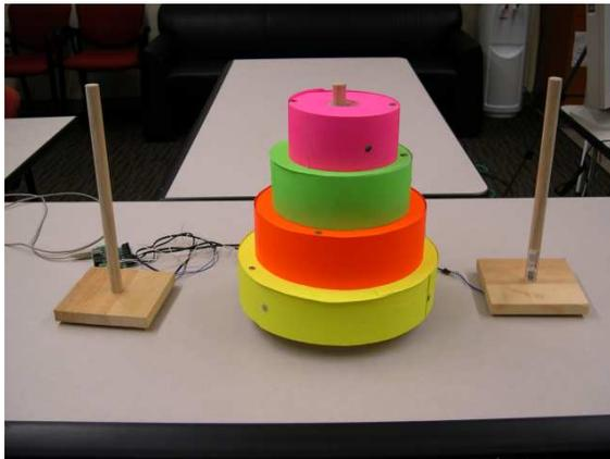
Fig. 4. The classic Towers of Hanoi puzzle with four rings and three pegs as used in the experiments. In our set-up, each of the three rings has a different color and mass. Weight sensors under each peg and a single camera allow the robot to estimate the state of the puzzle.
