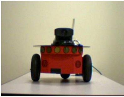
Fig. 1. The ActivMedia Pioneer 2 DX robot used in the experiments, as seen in the remote robot setting. The motions of the PTZ camera provide feedback that supplements the audio.
