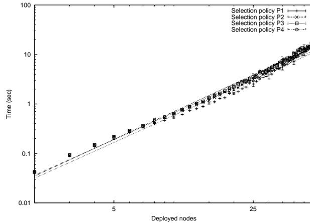
Figure 6. Assignment time (CPU) for policies P1 to P4. The scale is log-log. Most of the error bars have been suppressed for the sake of clarity.
