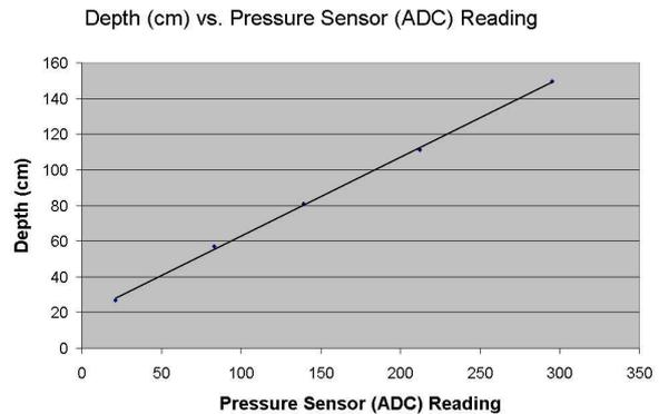
Fig. 7. Depth vs. Pressure Sensor (ADC) Reading
