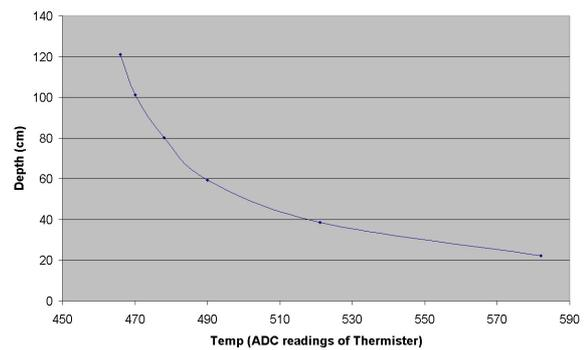
Fig. 8. Depth (cm) vs. Temperature (ADC Readings of Thermistor)
