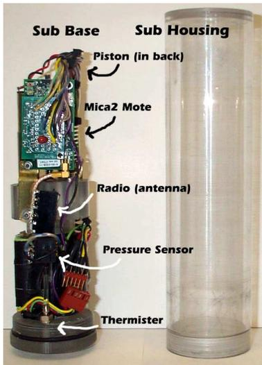
Fig. 2. The robot base and waterproof housing
