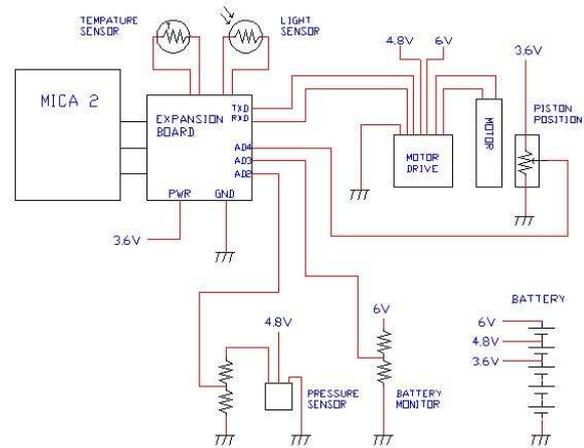
Fig. 3. Circuit schematic of the robot
