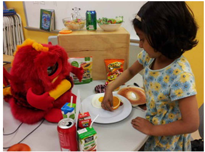
Fig. 1. An example of a socially assistive robot. Chili, a squash-and-stretch 6 degree-of-freedom robot with a digital face, was used to interact with 5- to 8-year-old first graders to teach and motivate them to make healthy food choices. The study involved 26 children interacting with the robot twice per week for 3 weeks and found that the children learned nutrition concepts and engaged with the robot and that their verbal responses to the robot became richer over time.
