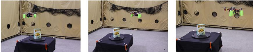
**Fig. 4** Quadcopter experiment and test setup. The quadcopter robot, equipped with a RGB-D camera, collects multiple views of a target object (e.g., a cereal box) in an active object recognition task.
