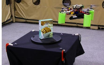
Fig. 1. Test setup for active multi-view object recognition and change detection. RESL quadcopter equipped with an ASUS Xtion RGB-D sensor, flying around a target object.
