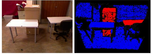
Fig. 5: Binary ground truth label of ‘pushable forward’. The left table in front of the box and the chair in front of the right table are ‘not pushable forward’ as there are objects behind them (red: pushable forward, blue: not pushable forward).
