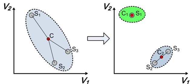
Fig. 6: Example step of iterative k-means clustering, with two label vectors  $V_1, V_2$ . Set  $S = \{S_1, S_2, S_3\}$  is split into two subsets by k-means clustering and the entropies are computed from the centroids of the sets. If  $H(C) > H(C_1)$  or  $H(C_2)$ , subsets are iteratively split again.
