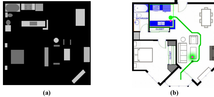
Fig. 3. (a) Pragmatic field indicating suitable surfaces for object placement (weight values in grayscale); (b) Task solution for “Take the cup to the kitchen” incorporating pragmatic constraints, with combined semantic/pragmatic field shown at object placement location
