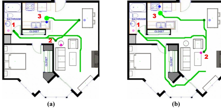
Fig. 4. Robot execution paths for test runs (a) Run #1 (no constraints) (b) Run #2 (constraints)
