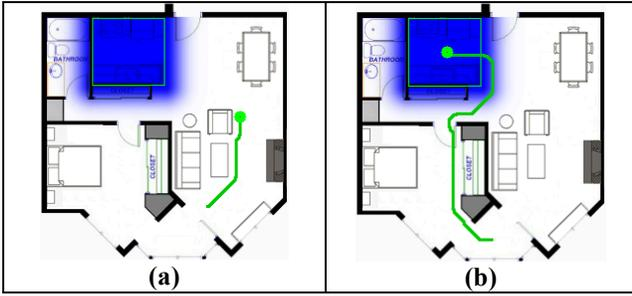
Figure 1. Two example paths for “to the kitchen”. (a) Path value =  $1.8 \times 10^{-10}$ ; (b) Path value = 1.0. Note:  $\sigma = \text{robot width} \times 2.5$
