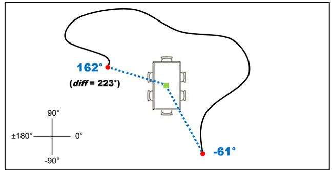
Figure 3. Path traveling around a dining table reference object, showing start and end orientations, with resulting *circumcentric* semantic field value =  $|223^\circ|/360^\circ = 0.61944$ .
