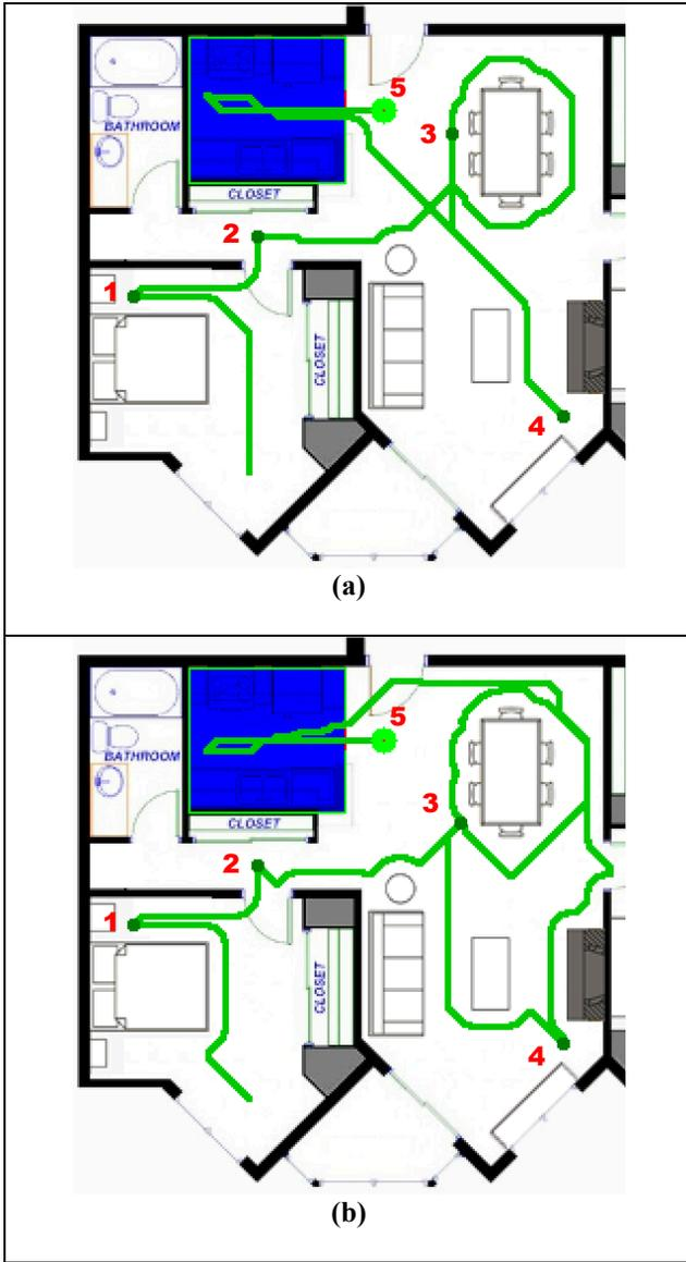
Figure 5. DSR path generation results for entire instruction sequence with and without user-specified constraints. (a) Test Run #1 (no constraints); (b) Test Run #2 (constraints). Note: path endpoints for each instruction are labeled with the instruction number.
