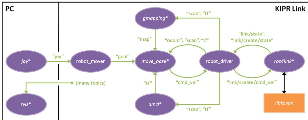
Figure 3: The distributed network of ROS nodes for our example system. Note that some nodes, connections, and other details are omitted for clarity.
