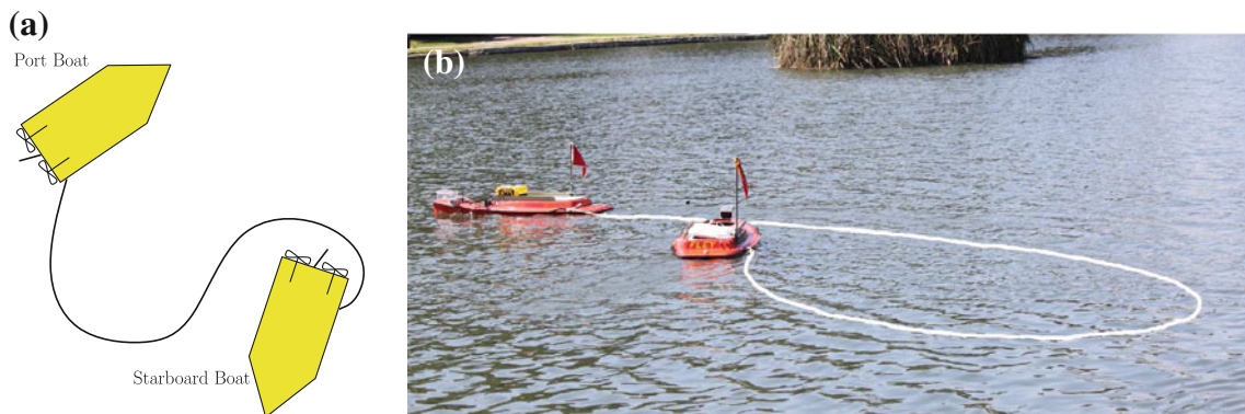
Fig. 6 a Sketch of the twisted rope situation. b Twisted condition with the real vehicles. The rope in the picture is highlighted to easily recognize its shape
