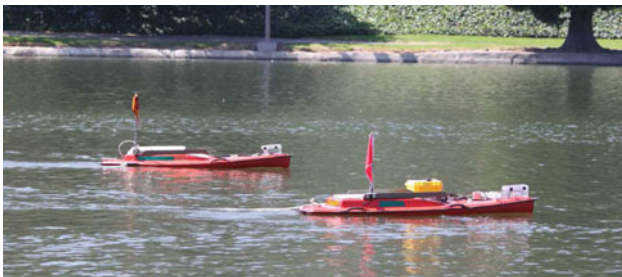
Fig. 11 The USC RESL Autonomous Surface Vehicles connected with a floating rope
