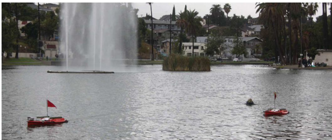
Fig. 1 Two autonomous surface vehicles cooperatively caging an object floating on a lake surface
