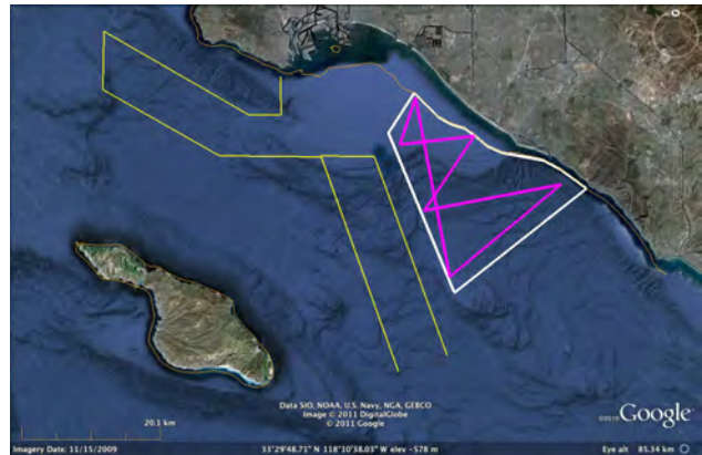
Fig. 1. General search area (white polygon) and predetermined path (magenta line) to be executed by an autonomous glider. The yellow lines denote the primary shipping lanes for Long Beach Port; areas that must be avoided. Image created by use of Google Earth
