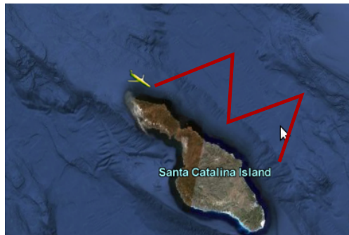
Fig. 1: Position and a planned path for one of our underwater gliders near Catalina island. We deploy the gliders in the Southern California Bight (SCB), to collect data including temperature, conductivity and salinity.
