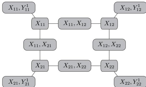
Fig. 2. The generalized cluster graph for approximate inference over  $\mathcal{H}_1$  in Fig. 1 [15].
