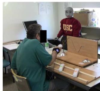
Fig. 2. The physical setup for the SAR rehabilitation experiments: Bandit humanoid robot, wire puzzle, wands, and wearable motion sensor.
