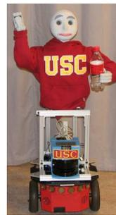
Fig. 1. Bandit, the humanoid robot used in our experiments.
