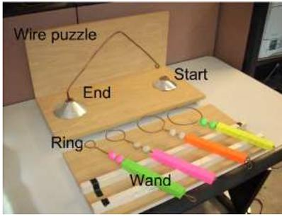
Fig. 3. The wire puzzle and wand setup. Wands of different difficulties are shown. Multiple puzzle shapes were also used. Participants guided the wand along the wire puzzle from Start to End, and back, attempting to avoid contact between the puzzle and the wand.
