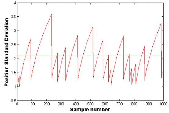
Figure 5: Illustration of position error standard deviation (shown in red) when walking at a self-selected speed for one trial run in the L-shaped trajectory. Similar plots are observed across other trajectories and both users. Regular correction from WiFi readings reduce process covariance. The mean standard deviation of position per experimental run was  $\approx 2.1$  m (shown in green).
