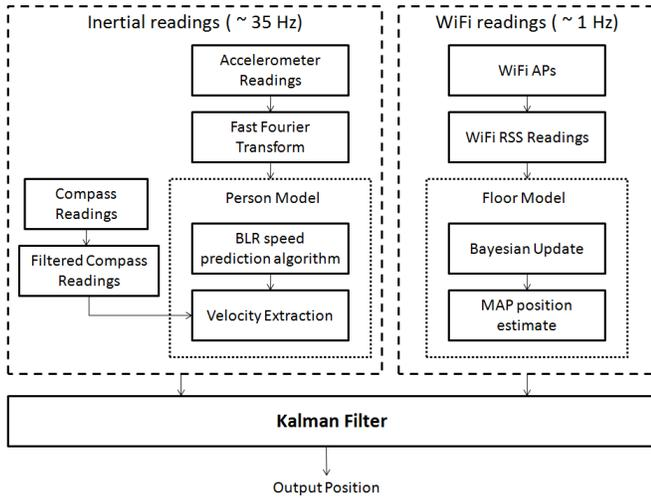
Figure 2: Illustration of the complete framework for trajectory prediction. Inertial and WiFi readings are fused using a Kalman filter. Inertial readings are converted to velocity measurements using the techniques outlined. Velocity measurements are used to propagate state (update step). For each WiFi reading, the location distribution is updated using Bayes rule and the MAP position estimate is taken from the distribution. This forms the correction (measurement step).
