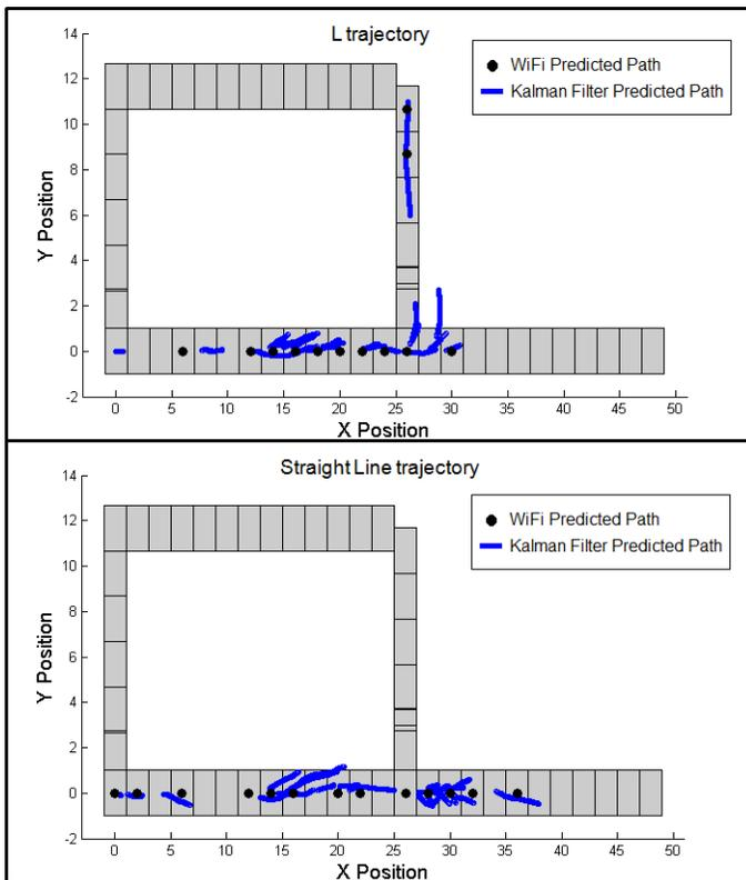
Figure 6: Illustration of predicted trajectories using WiFi alone and with Kalman Filter fused measurements from inertial sensors. Regular correction from Wi-Fi helps prevent inertial sensor drift.
