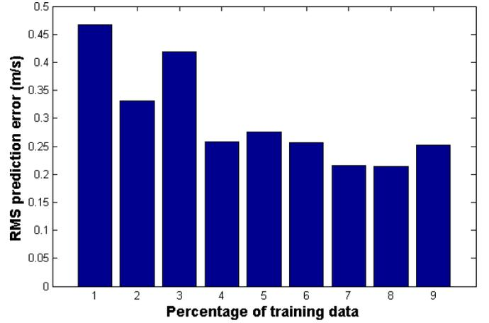
Figure 3: Illustration of errors obtained from user model with percentage of training data available. Errors reduce with increasing amount of training data. Least average error is  $\approx 0.2 - 0.25$  m/s. This corresponds to an average distance error estimate of  $\approx 6 \times 10^{-3}$  m for each time instant.
