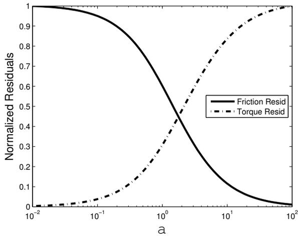
Fig. 5. Torque and friction residuals shown against  $\alpha$ .
