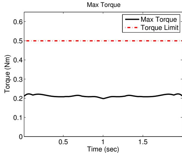
Fig. 7. Maximum joint torque during four-fingered simulations described in Section IV-B.1.
