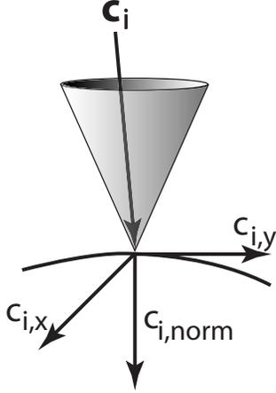
Fig. 2. A contact point showing the contact force vector,  $\mathbf{c}_i$ , its normal and tangential components, and the Lorentz cone within which the contact vector must reside.
