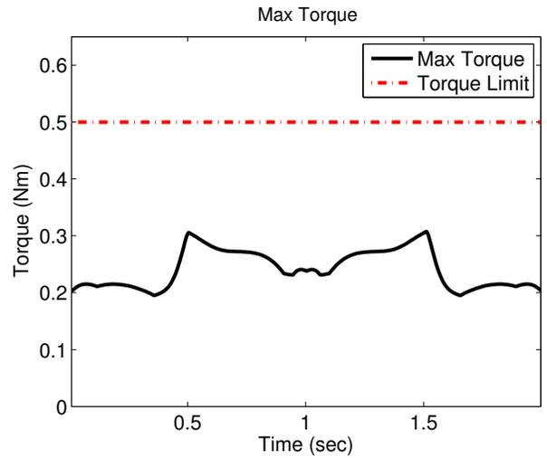
Fig. 10. Maximum joint torque during regrasping simulations described in Section IV-B.2.
