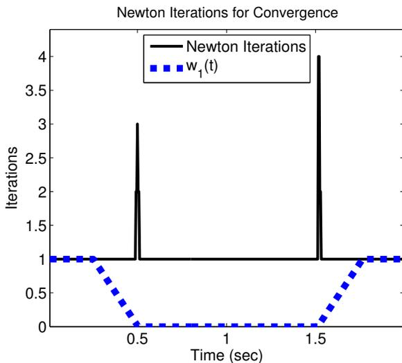
Fig. 12. Newton iterations required for convergence shown with  $w_1(t)$  during simulated execution of a test trajectory.
