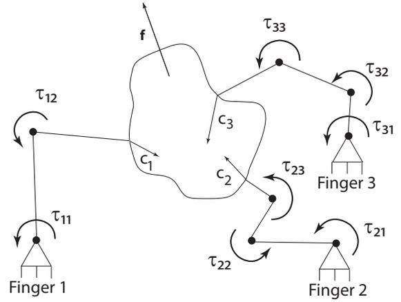
Fig. 1. A three-fingered hand grasping an object. Joint torques,  $\tau_{ij}$ , contact forces,  $\mathbf{c}_i$ , and the desired wrench,  $\mathbf{f}$ , are shown.
